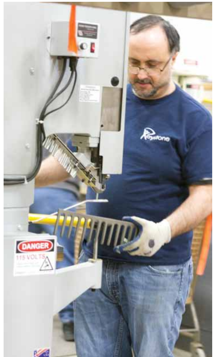
John using an Orbitform riveter to attached the head of a rack to the handle.
