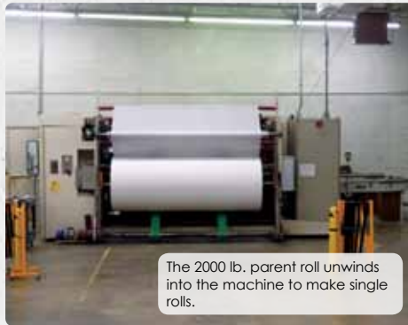
The Perini 716B machine unwinds, perforates, and cuts toilet paper logs into single rolls.
